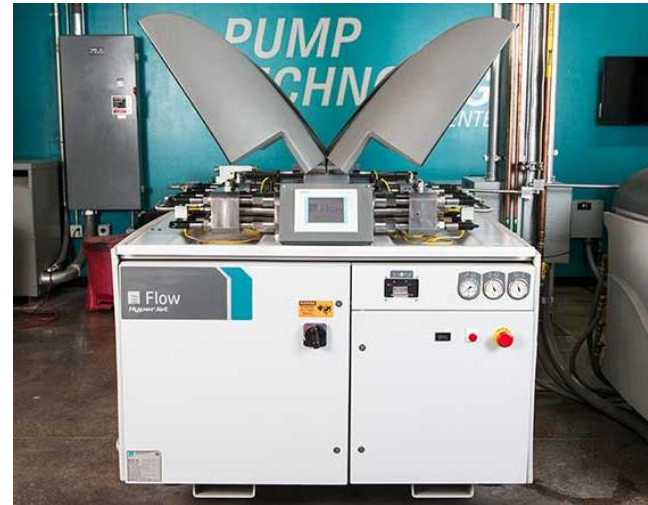
Linear Intensifier Pump Rated up to 94,000 psi [6,500 bar]
